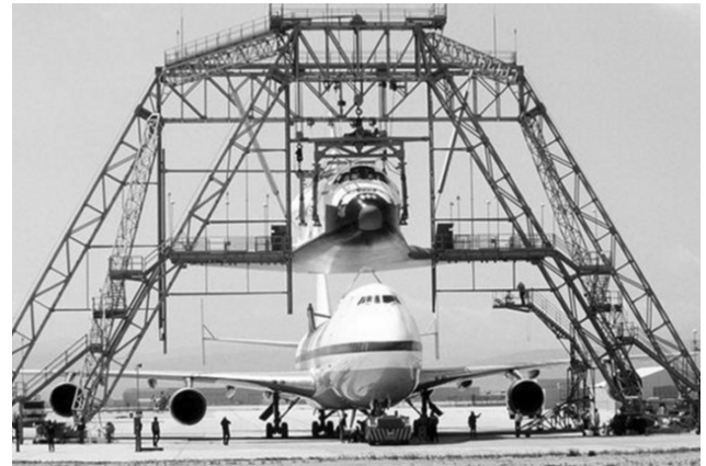
Fig. 3 747 Shuttle ferry aircraft and orbiter in loading tower.
