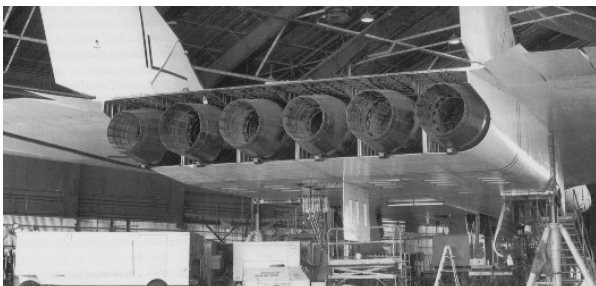
Fig. 11 YJ93-GE engines of XB-70.
