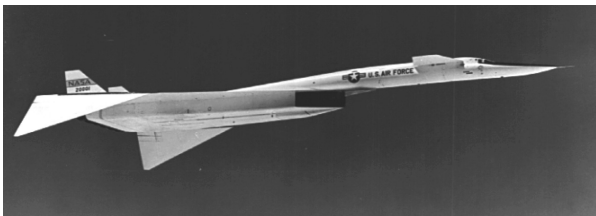
Fig. 10 XB-70: Mach 3.1 with conventional turbojet propulsion.
